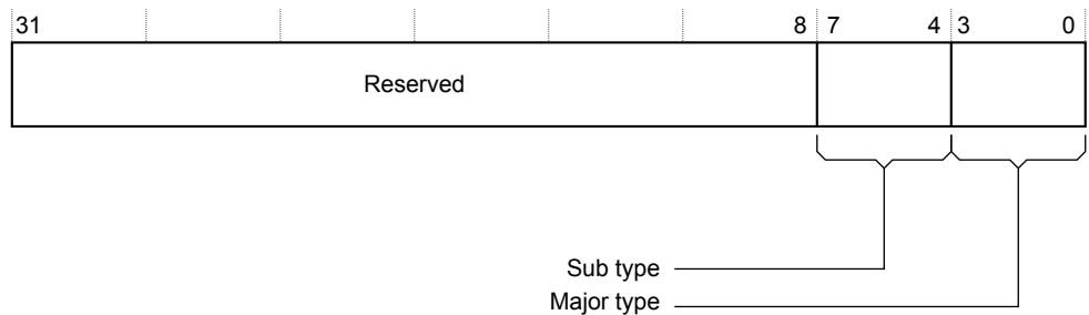
Figure 11-12 TPIU_DEVTYPE bit assignments
