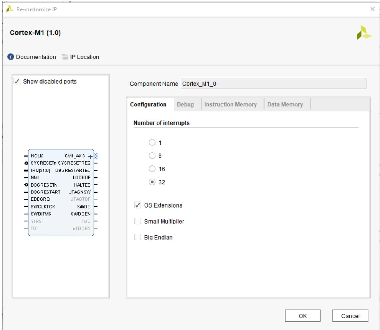
**Figure 3-1 Configuration tab**
