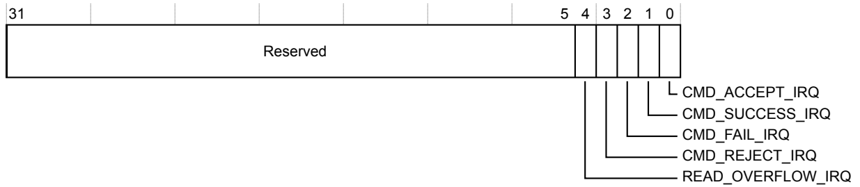
Figure 3-10 IRQ_MASKED_STATUS register bit assignments
