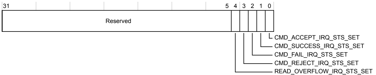
Figure 3-8 IRQ_STATUS_SET register bit assignments
