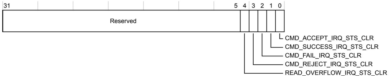
**Figure 3-9 IRQ\_STATUS\_CLR register bit assignments**
