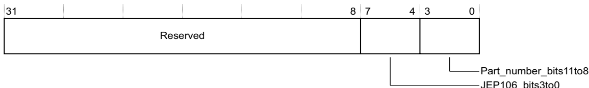
Figure 3-22 STMPIDR1 Register bit assignments
