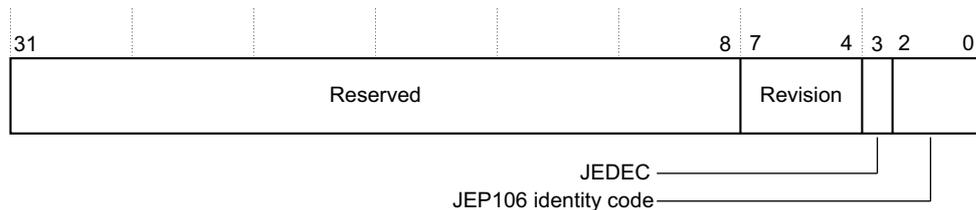
Figure 3-20 PeriphID2 register bit assignments
