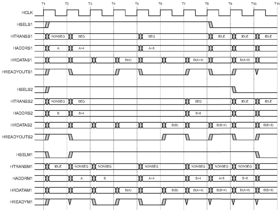
Figure 8 Parallel access timing diagram
