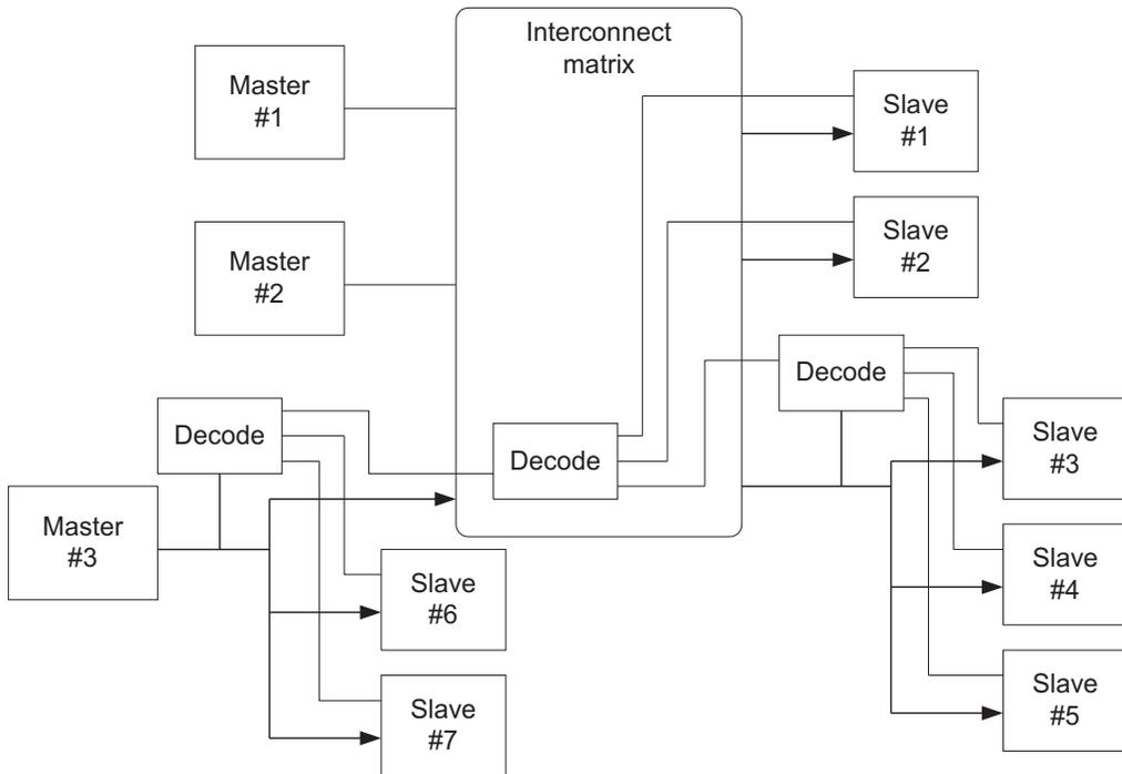
**Figure 7 Address decode**
